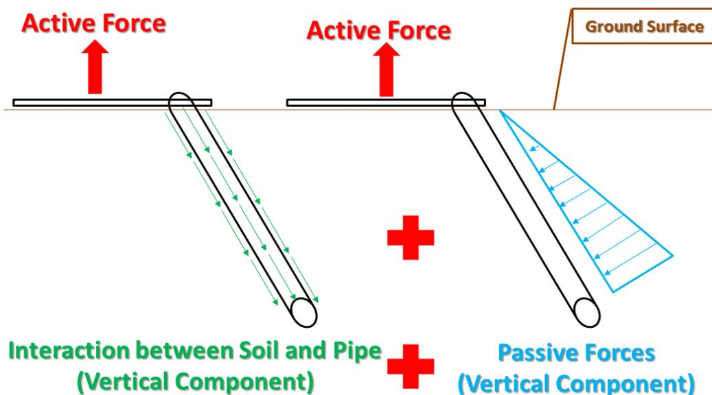
Figure 21: Resisting forces against the uplift or pull-out forces
