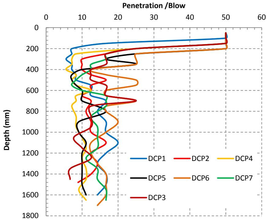
Figure 9: DCP results in terms of penetration (mm) per blow against depth
