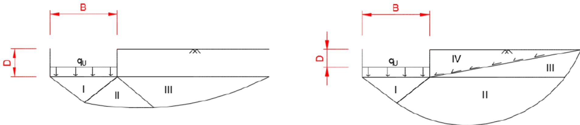
**Figure 2: Soil movement and failure pattern; Terzaghi (left); Meyerhof (right)**
