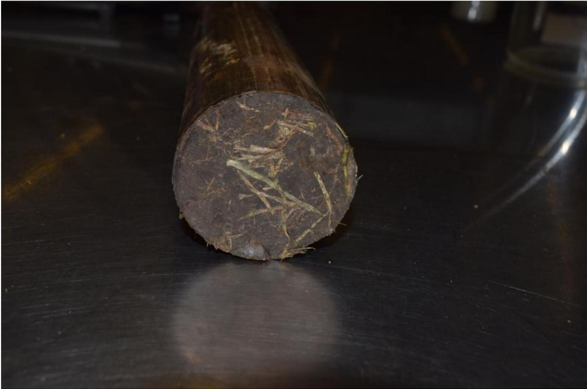
Extracted clay specimen from Shelby tubes
