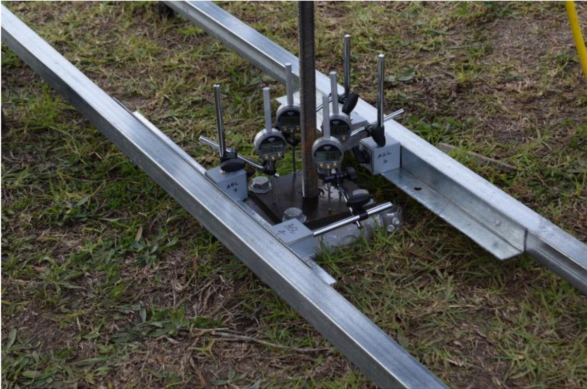
LVDTs and the mounting beams for pull-out tests
