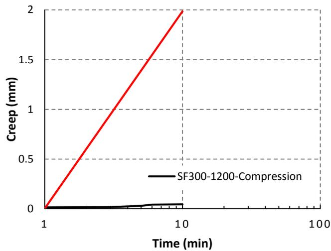
Figure 16: Compression test result for SF300-1200
