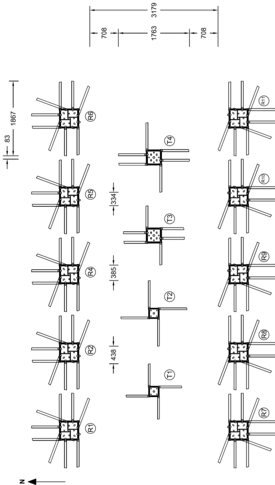
Figure 7: Layout of Surefoot footings and orientation of micropiles (dimensions in mm)
