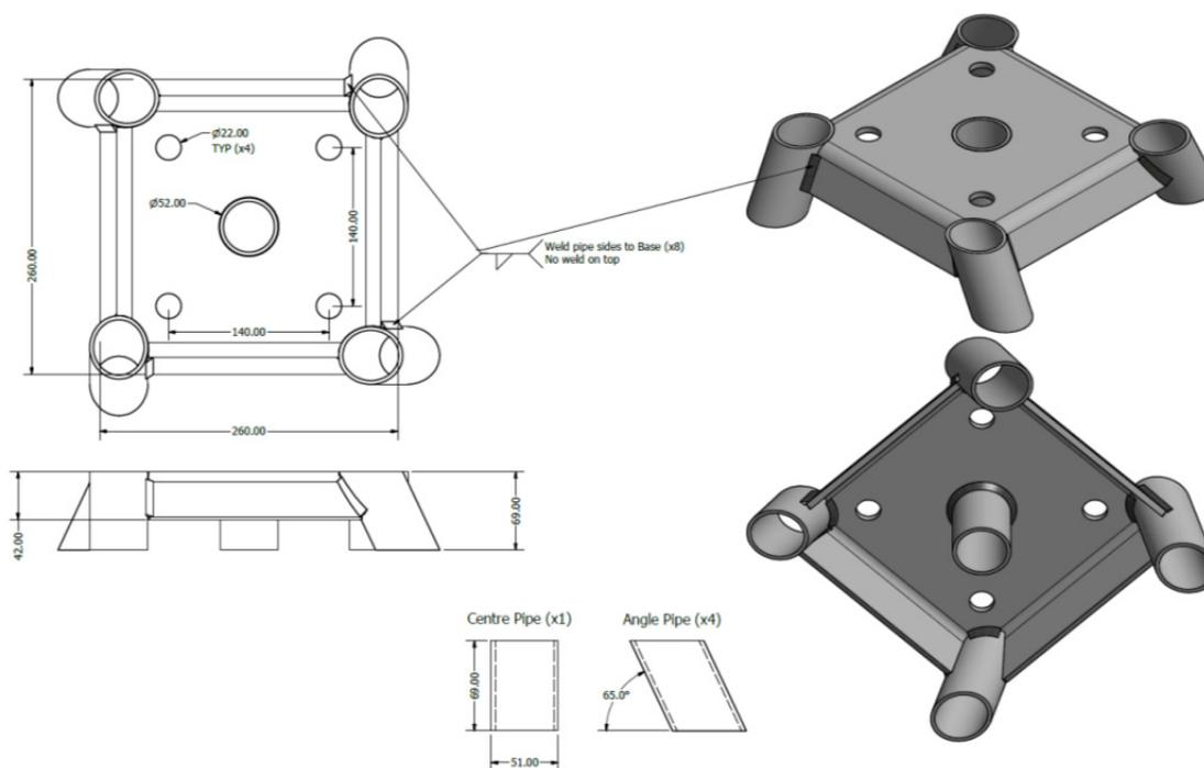
Figure 2: Surefoot SF100 dimensions (in mm) and details
