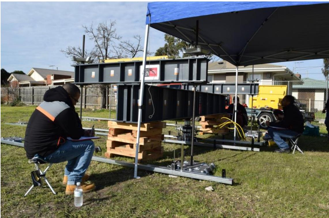
Reading reaction piles movement on each side
