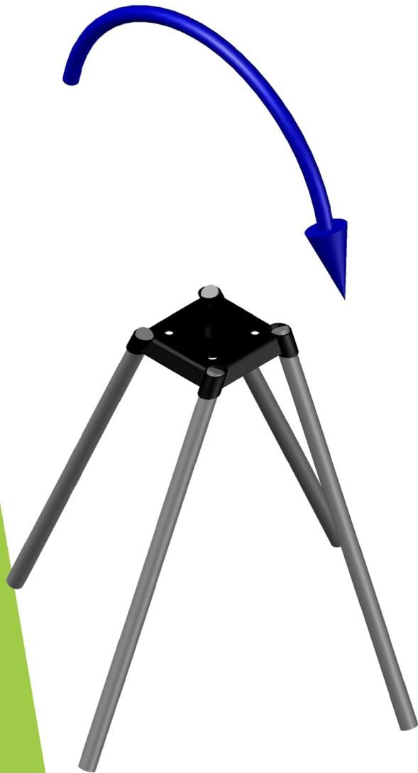
Since the bending moment applied transforms into a pair of forces, and the difference in the capacity between piles under compression load and piles under tension load is wide, it is more conservative to disregard the effect of piles under compression and only design the bending moment being resisted by the piles under tension loading, with a new neutral axis now closer to the compression side.
