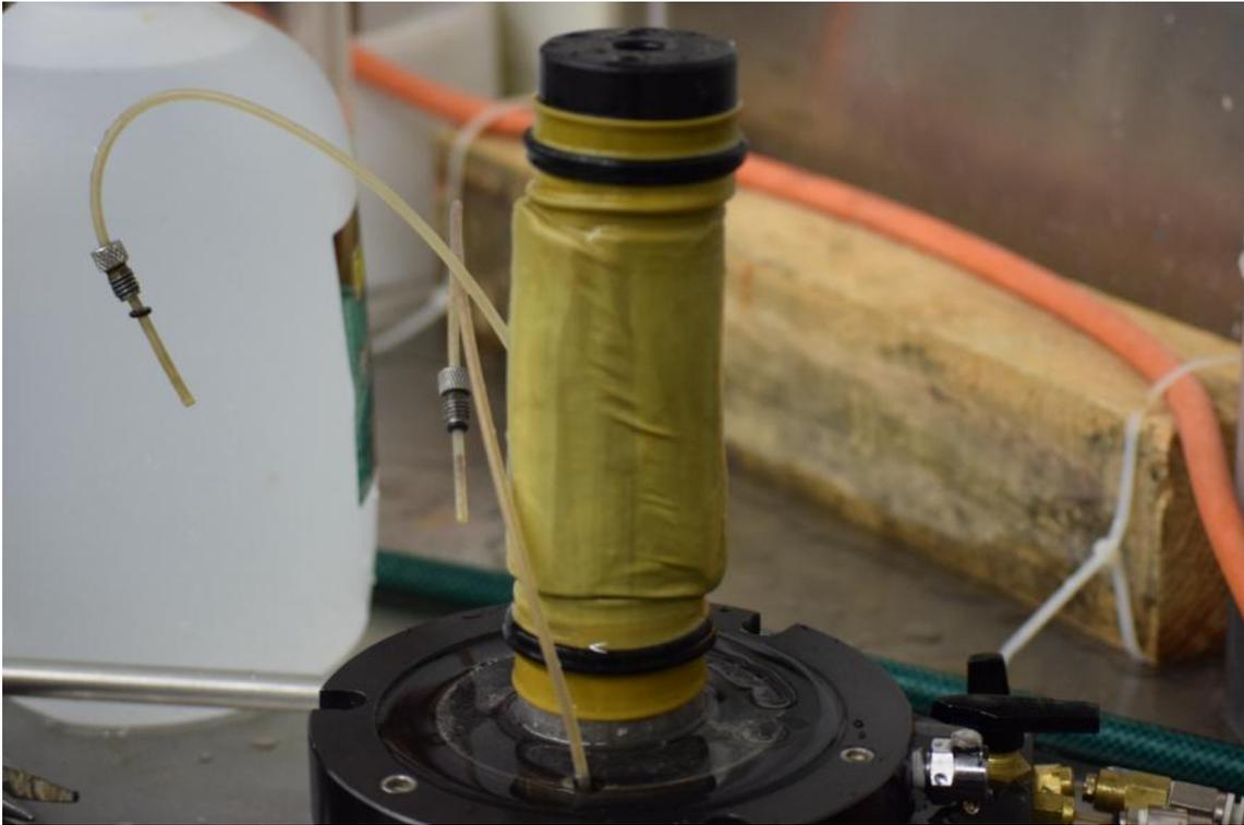
**Braybrook clay specimen after triaxial shear strength test**
