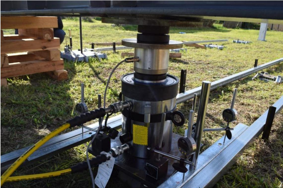
Hydraulic jack, load cell, ball bearing and LVDTs
