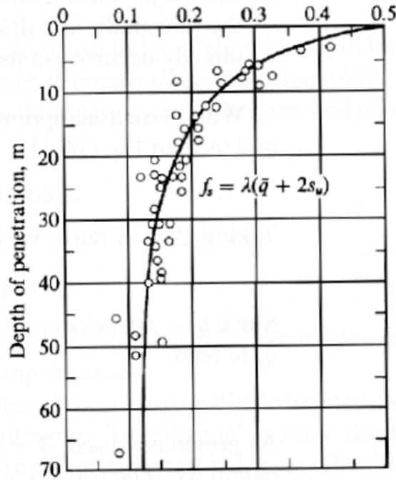
Figure 22. Variation of  $\lambda$  with pile embedment length (Das, 1995)
