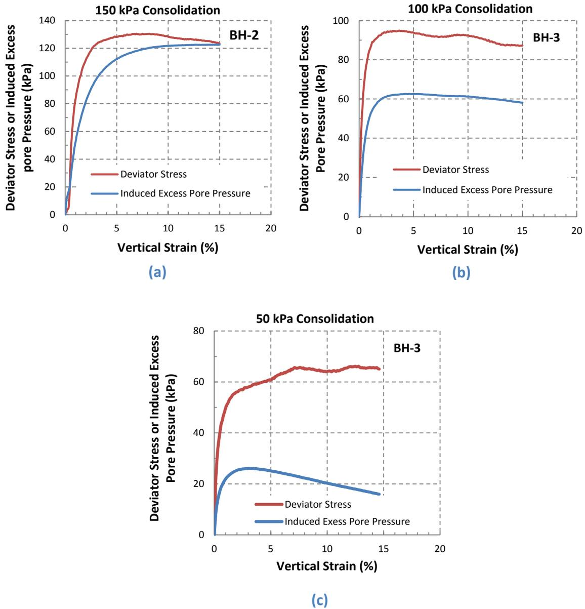
Figure 11: Deviator stress and induced excess pore pressure from the CU triaxial test for (a) BH-2, 0.9-1 m, (b) BH-3, 0.5-0.6 m and (c) BH-3, 0.8-0.9 m
