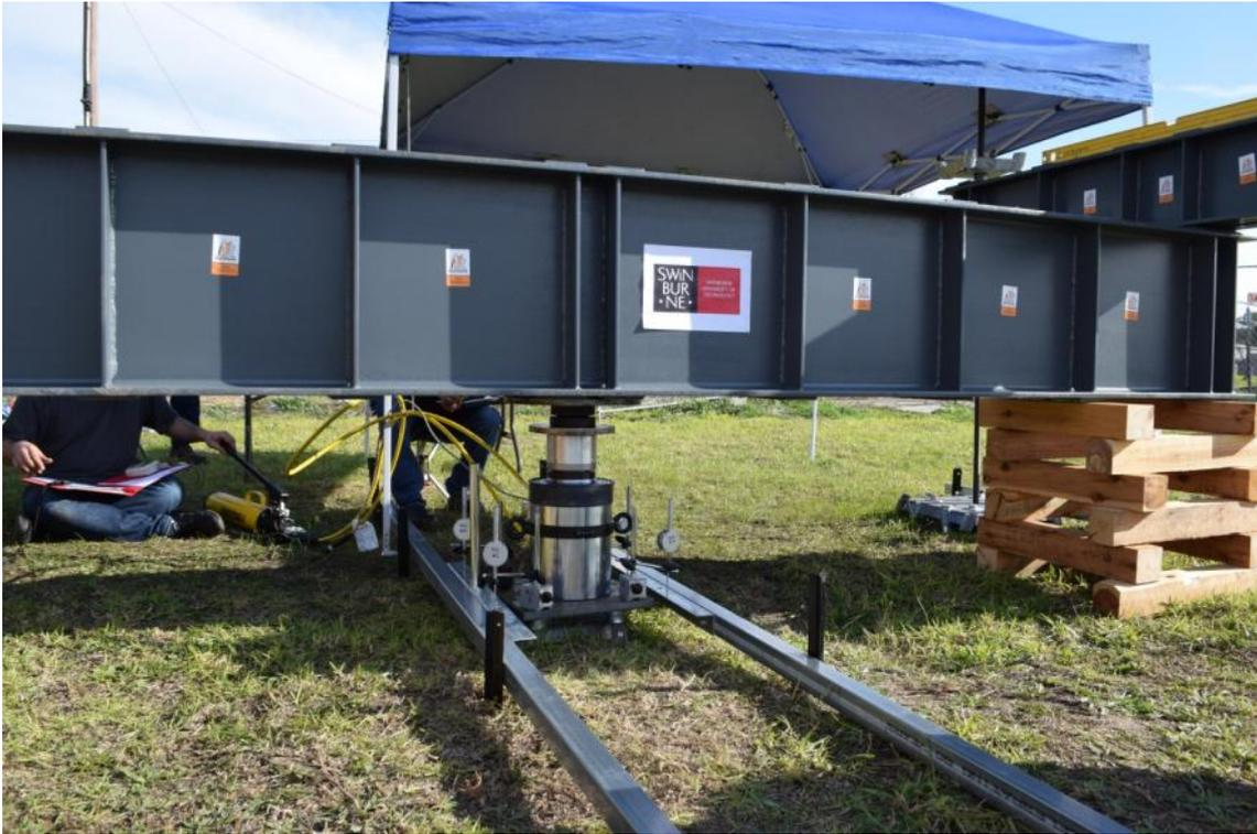
Hydraulic loading system and LVDTs mounting beams
