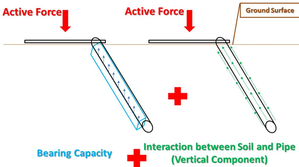
Figure 20: Resisting forces against the gravity active forces
