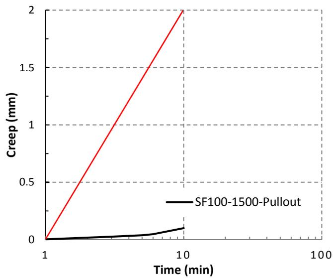
**Figure 15: Pullout test result for SF100-1500**
