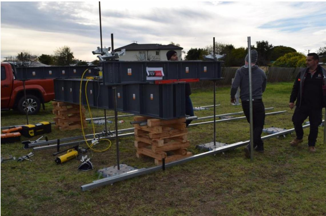
Beam seating on timber cribs for pull-out test
