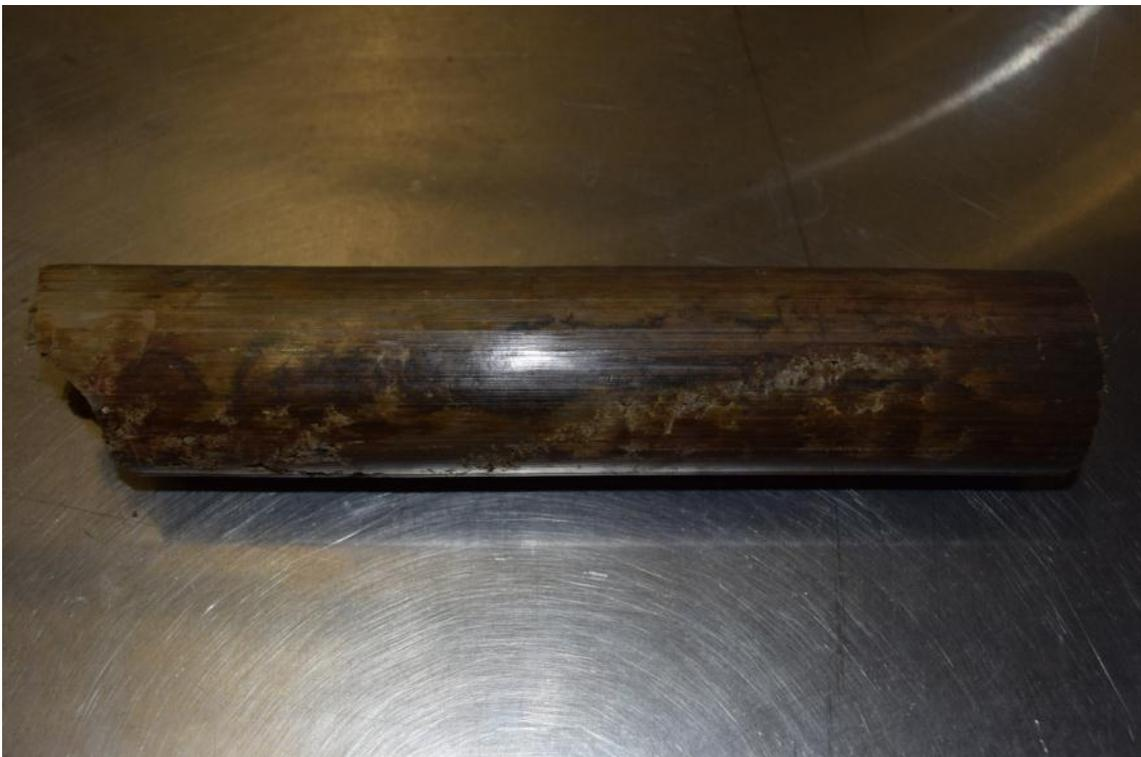
Extracted clay specimen from Shelby tubes
