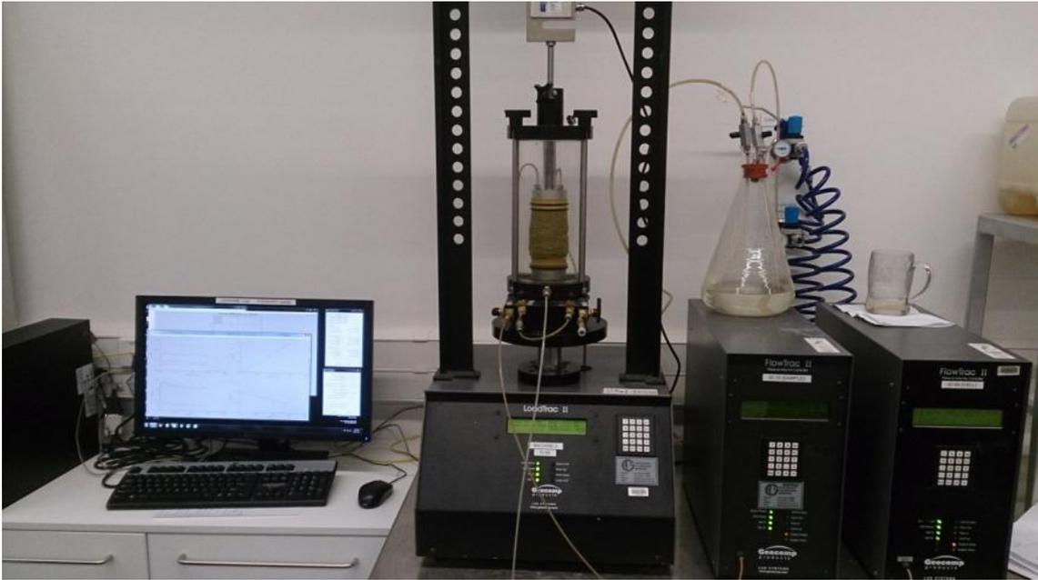
Automatic triaxial system during testing
