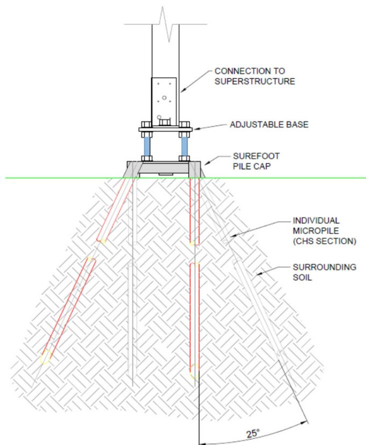
**Figure 1: A typical Surefoot system with surrounding soil and connections**
