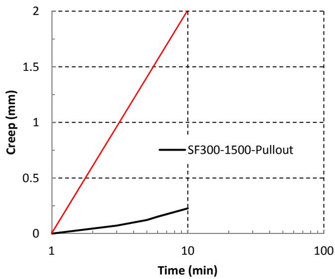
**Figure 19: Pullout test result for SF300-1500**
