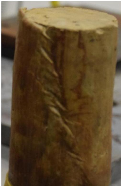
**Failure band on triaxial specimen of Braybrook clay**
