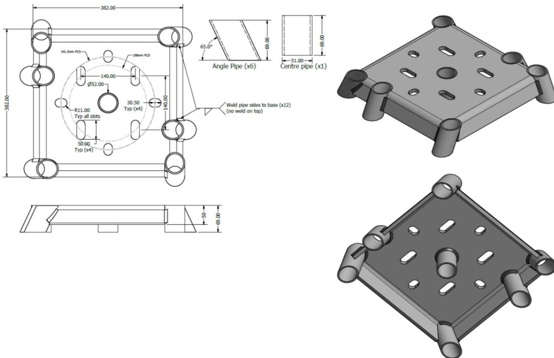
**Figure 3: Surefoot SF300 dimensions (in mm) and details**
