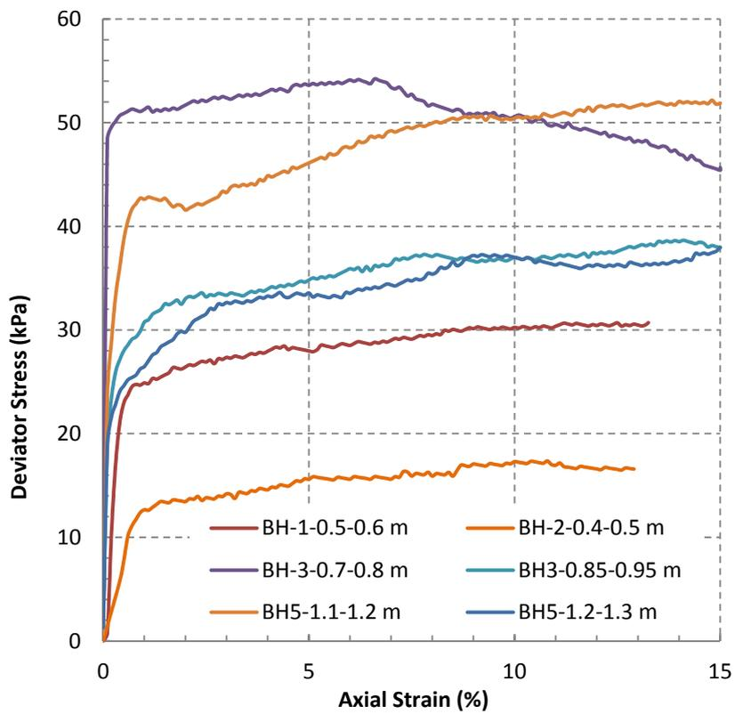
Figure 10: Deviator stress vs axial strain from UU triaxial tests
