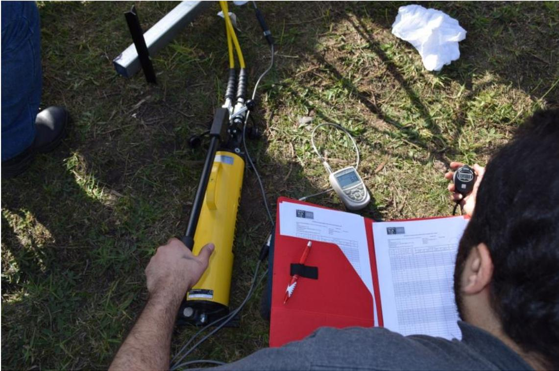
Hydraulic loading system and load cell screen
